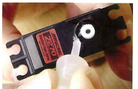
Some servos are sealed, but a little extra protection can't hurt.
