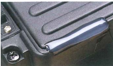
A little grease between the receiver box and the lid is a sure way to prevent water from entering. You may have to reapply the grease if you remove the cover.
