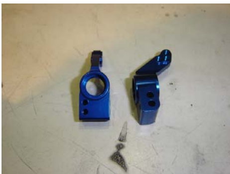
4352X : Stub axle carriers, blue-anodized 6061-T6 aluminum, rear (1.5 degrees toe-in)(L&R)
